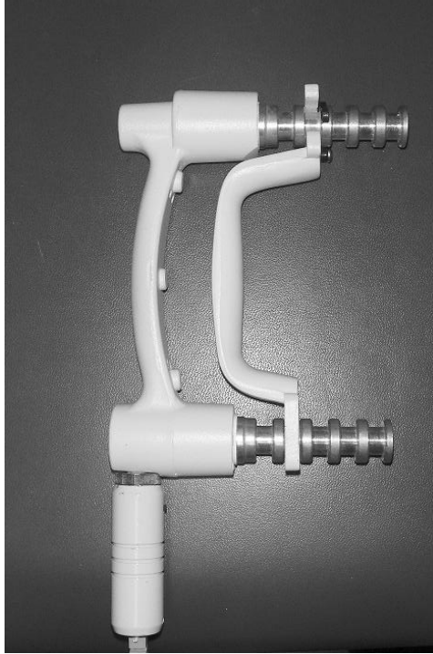
Figure 1. Modified hand grip dynamometer
